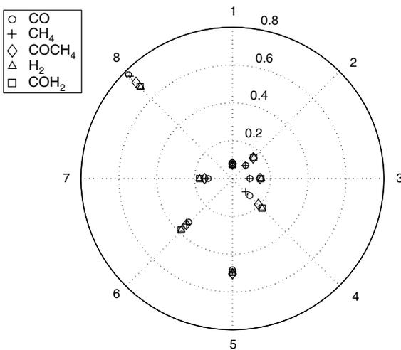
Fig. 4. Polar representation of the array response exposed to different gases. Measurement type, CO (circles), CH<sub>4</sub> (plus signs), mixture CO–CH<sub>4</sub> (diamonds), H<sub>2</sub> (triangles) and mixture CO–H<sub>2</sub> (squares).
