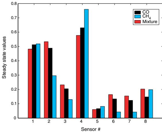
Fig. 3. Histograms showing the response patterns of the eight gas sensors exposed to CH<sub>4</sub>, CO and their mixture.
